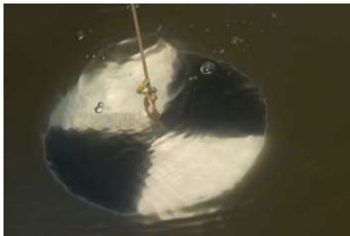
Figure 10: Black and white Secchi disk
