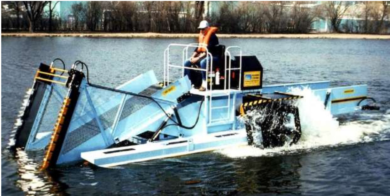
18 Figure 33 – Aquarius Systems EH-220 Aquatic Plant Harvester with a 5-ft cutting blade and 210 cu.ft 19 cut material storage 20
